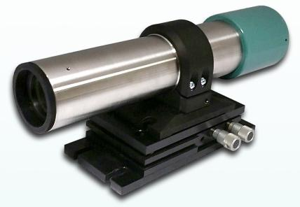
Electronic Autocollimator is equipped with a USB 2.0 camera of high resolution and allows the precise measurement of an angle position of moving and stationary objects.
